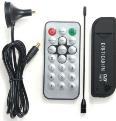
Fig. 14. The USB device used in our experiments, a DVB-T+DAB+FM device, with the Realtek, RTL2838UHIDIR, chipset.
