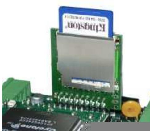
Double SD Card connector for Baseio ([schematic](#)).
