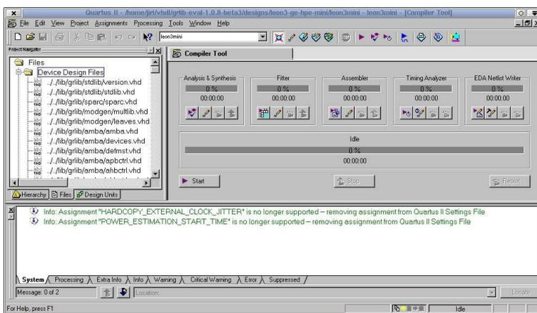
GRLIB includes a `leon3` template design for the HPE-Mini board from Gleichmann Electronics. The template design is located `designs/leon3-ge-hpe-mini`, and uses board settings from the `boards/ge-hpe-mini` directory. The `leon3-ge-hpe-mini` design can favorably be used a template for other Altera-based projects. It is essential that Quartus version 6.0 or later is used.
