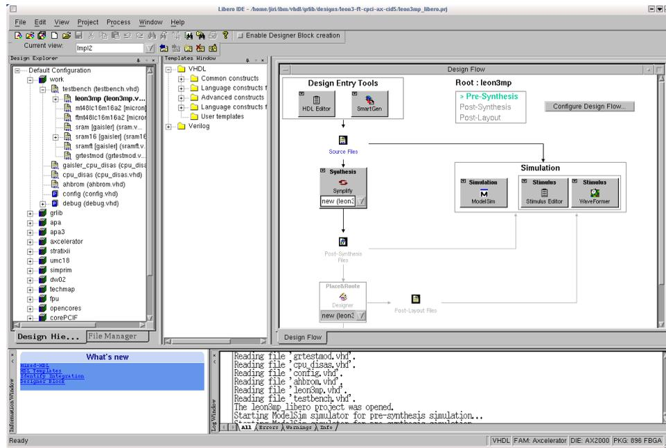
Note that when synplify is launched from Libero the first time, the constraints file defined in the local Makefile is not included in the project, and must be added manually. Before simulation is started first time, the file `testbench.vhd` in the template design should be associated as stimulyfy file.
