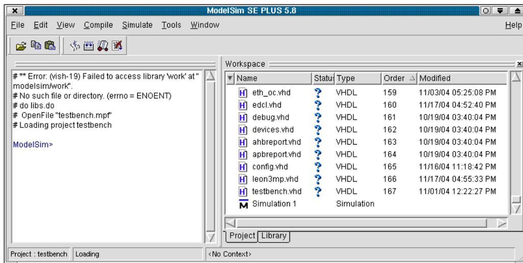
Figure 3. Modelsim simulator window using a project file
