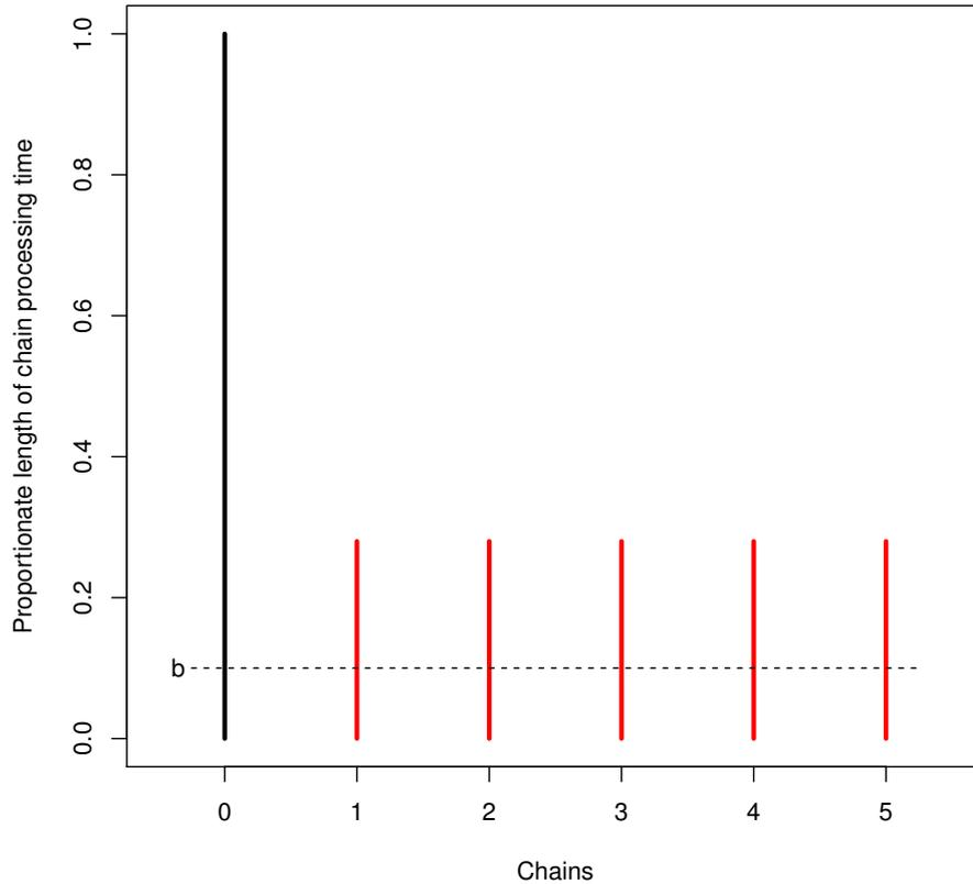
Figure 1: The theoretical gain due to multi-threading can be calculated by Amdahl’s Law. Let  $b$  be the burn-in fraction and  $C$  be the number of threads, then the gain limit is  $((1 - b)/C + b)^{-1}$ . In this diagram, the burn-in fraction,  $b = \frac{100}{1100} = 0.09$ , and the number of CPUs,  $C = 5$ , results in an elapsed time of only  $((1 - b)/C + b) = 0.27$  or a  $((1 - b)/C + b)^{-1} = 3.67$  fold reduction which is the gain in efficiency.
