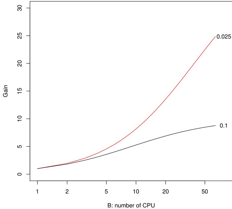
Figure 2: The theoretical gain due to multi-threading can be calculated by Amdahl's Law. Let  $b$  be the burn-in fraction and  $C$  be the number of threads, then the gain limit is  $((1 - b)/C + b)^{-1}$ . In this figure, the theoretical gains are on the y-axis and the number of CPUs, the x-axis, for two settings:  $b \in \{0.025, 0.1\}$ .
