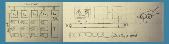
2 symmetric wires (twisted pair), GND + VCC. Termination resistors for reflection absorption.
